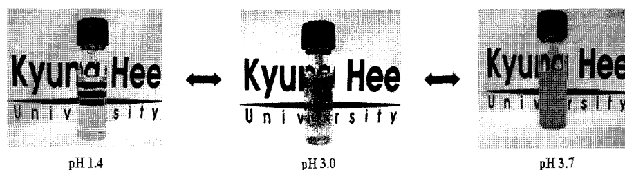
Figure 4. Photo image change of poly(ethylene oxide- b -maleic acid) obtained from the THF-insoluble fraction in aqueous media with pH (3.7 wt%).
