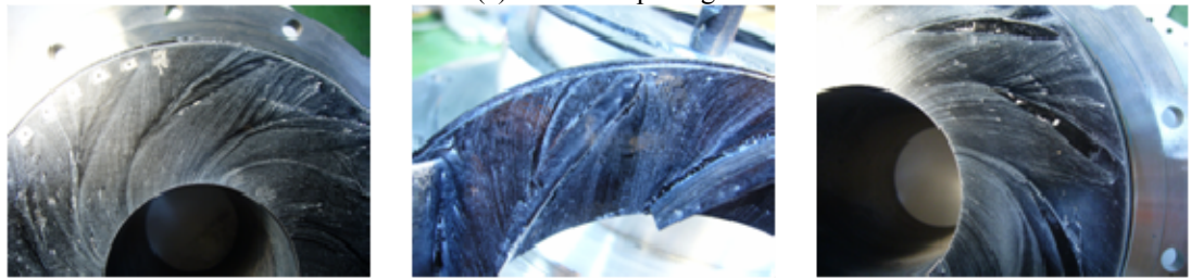
Shroud side (with clearance) Hub side (with clearance) Shroud side (without clearance) (b) Largest opening
