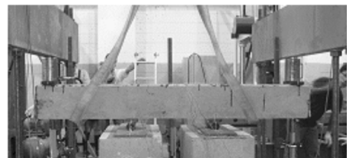
(b) Flexural test in progress
