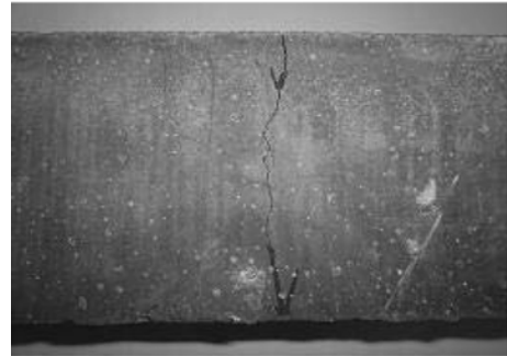
Fig. 10 Fracture pattern of NRCC
