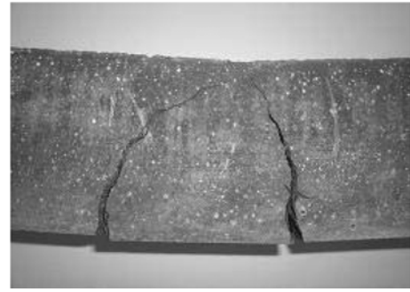
Fig. 9 Fracture pattern of RCC
