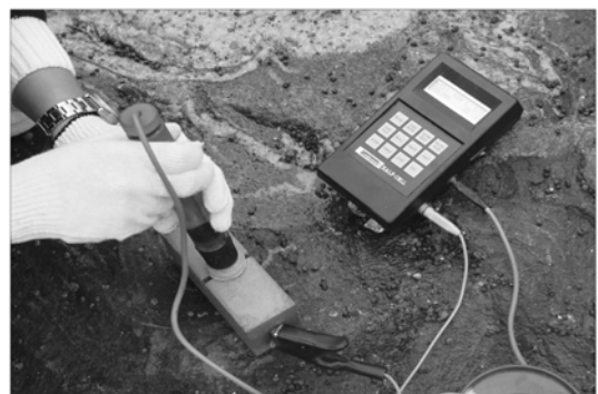
Fig. 8 Test of half cell potential
