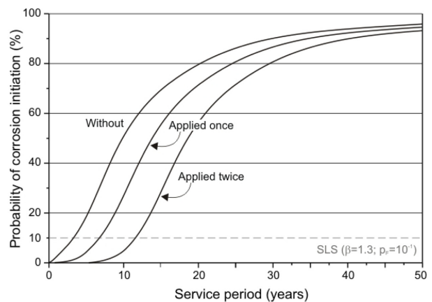
Fig. 8 Influence of hydrophobation coatings on the probability of corrosion initiation.
