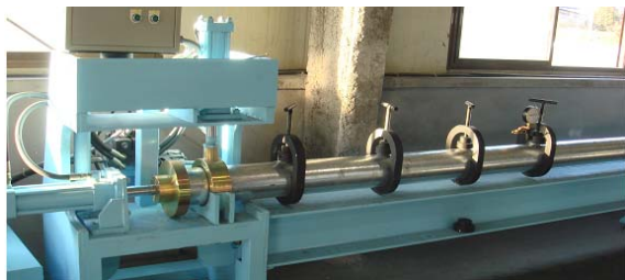
Fig. 15 Body strength test of TBP(150A×65, 80, 100, 125)
