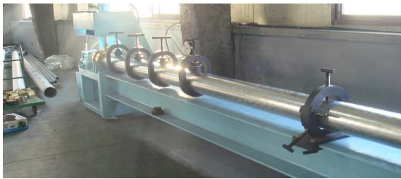
Fig. 14 Body strength test of TBP(150A×25, 32, 40, 50)
