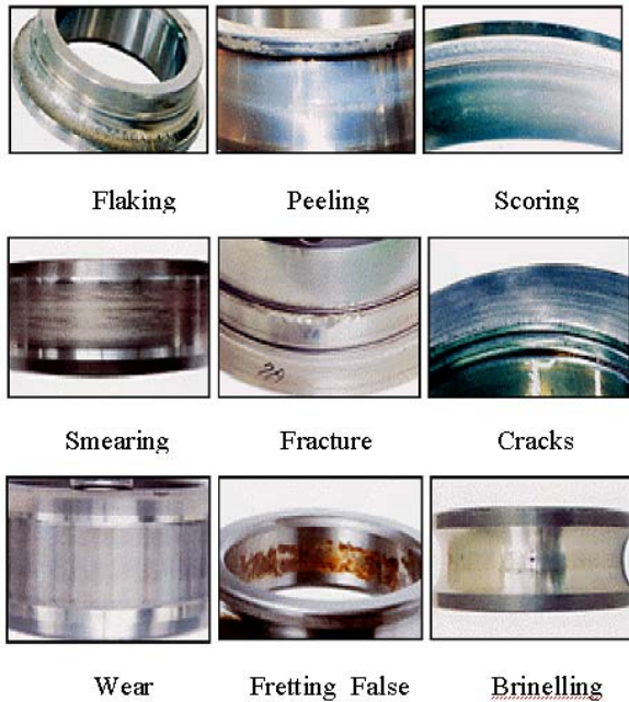
Fig. 1 Bearing failure types
