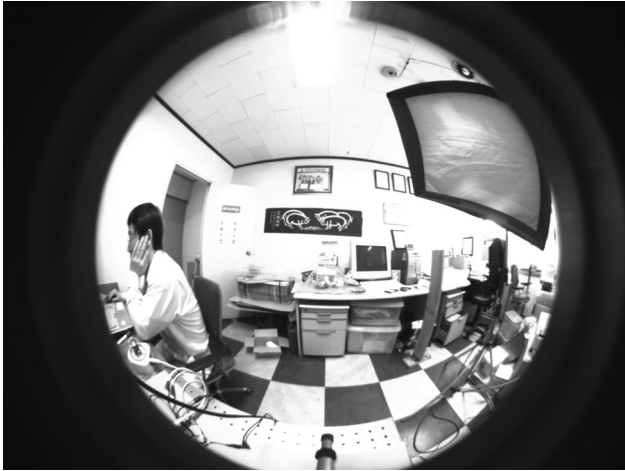
FIG. 14. A sample image of an office interior obtained using the developed fisheye lens.
