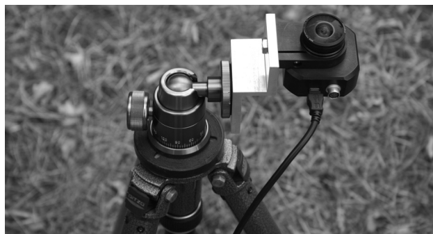
FIG. 11. An experimental setup to take a whole sky view using the developed fisheye lens.
