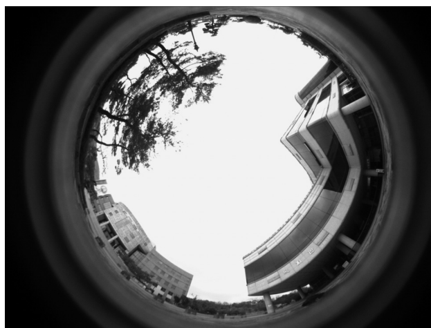
FIG. 12. A whole sky view obtained using the developed fisheye lens mounted on a 3M pixel CMOS camera.
