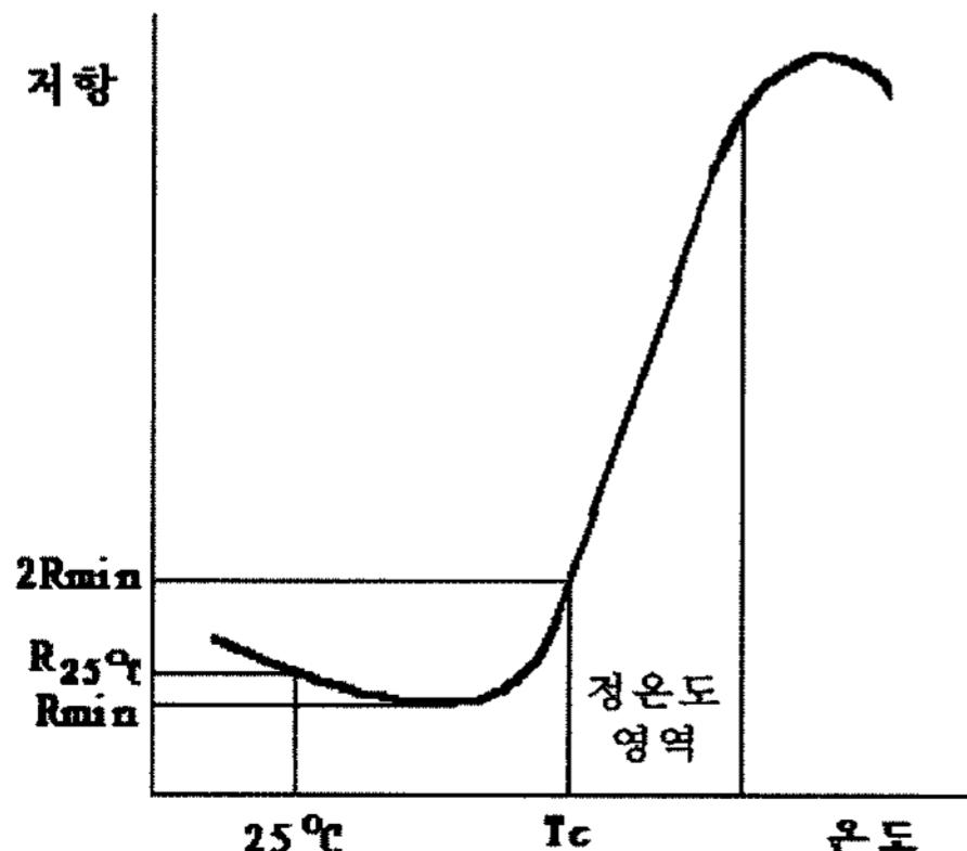
Fig. 2. Characteristic curve for resistance-temperature of PTC thermistor.
