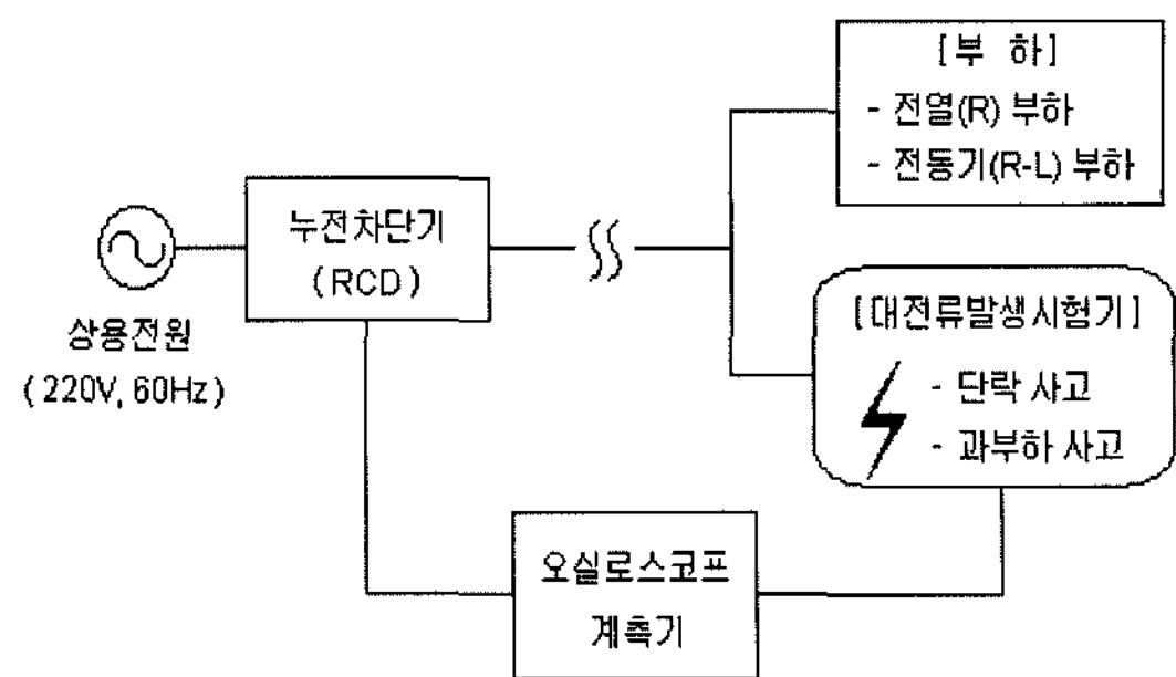
**Fig. 3.** Block diagram for performance analysis of RCDs.
