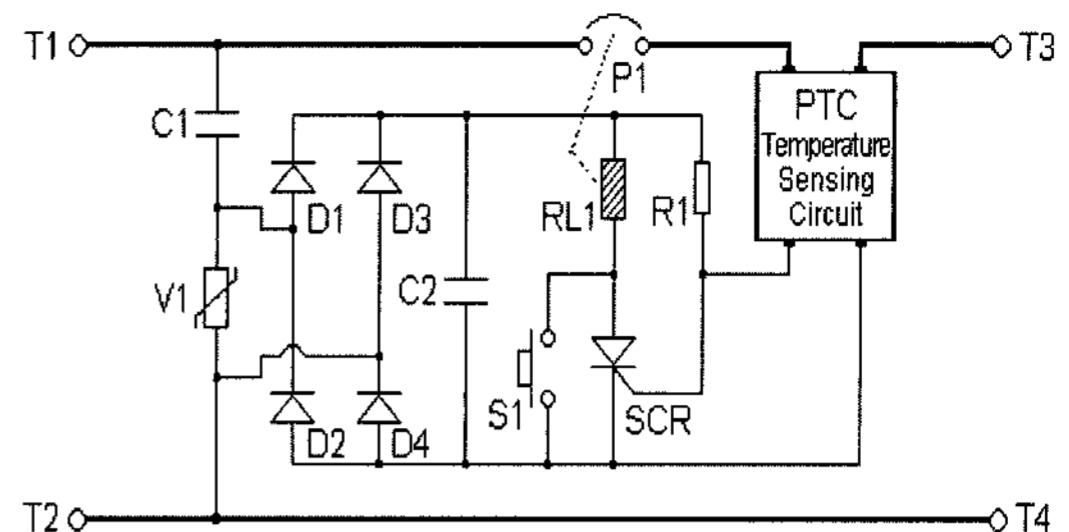
**Fig. 5.** Electrical fire prevention system by using PTC thermistor.
