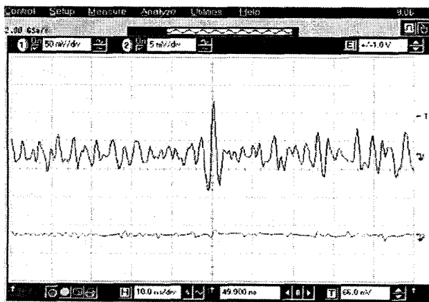
Fig. 3 Typical noise signal from the power system.
