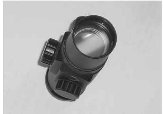
Fig. 8. Dot sight composed by the doublet reflector made from the data of Table 2.
