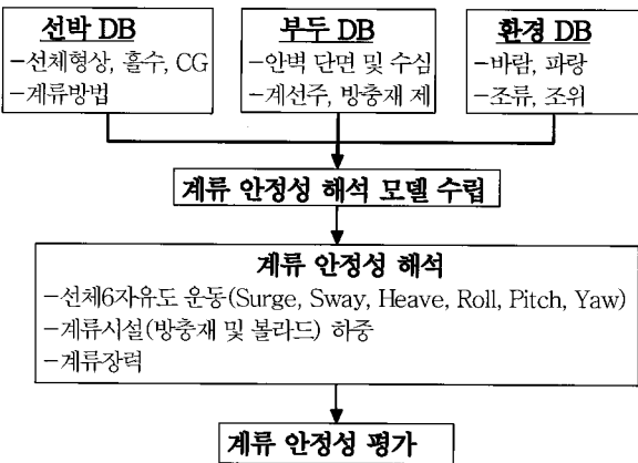
Fig. 2. Analysis and evaluation process of the mooring stabilities.
