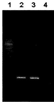
Fig. 2. Agarose gel electrophoresis of PCR products obtained after amplification of total DNA with the species-specific primers (EM1A, EM1B). Lanes 1, 500 bp DNA ladder; 2, E. faecium KCCM 12118; 3, strain JH95; 4, B. longum A24.
