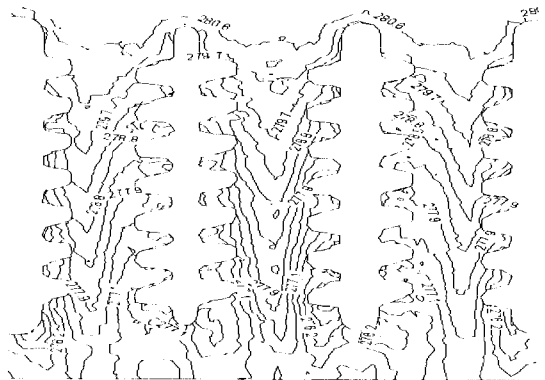
(b) Temperature contours of the bar(case 3)
