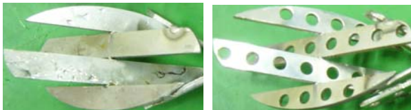
Fig. 3 Geometrical structure of unit element of SMXL-O and SMXL-H mixer
