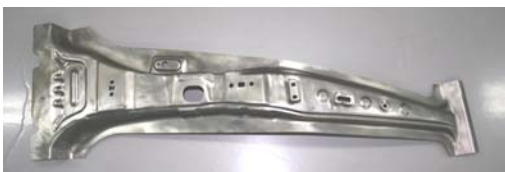
Fig. 6 Center-pillar panel made of boron steel for induction heating test
