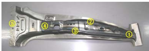
Fig. 9 Center-pillar panel after induction heating
