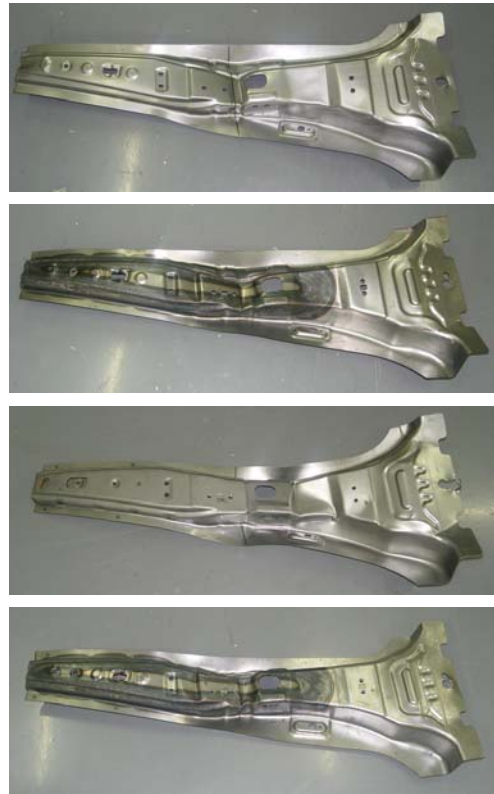
Fig. 14 Deformation result of each center-pillar specimen after static load test (From top; #1, #2, #3, #4)
