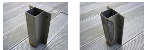
Fig. 4 Welded hat-shaped specimen with plate for static load test (Left; before induction heating, Right; after induction heating)
