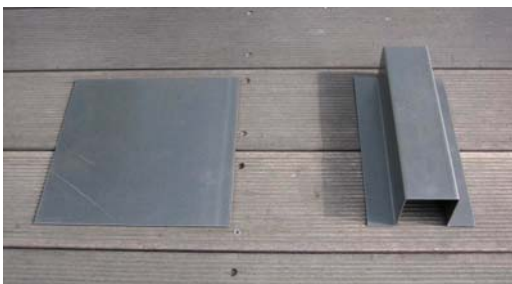
Fig. 1 Hat-shaped specimen for induction heating
