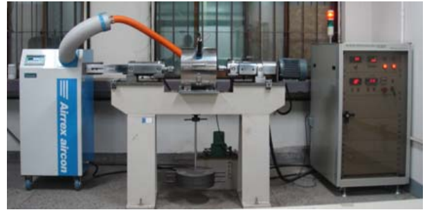
Fig. 3 Rotating bending fatigue testing machine
