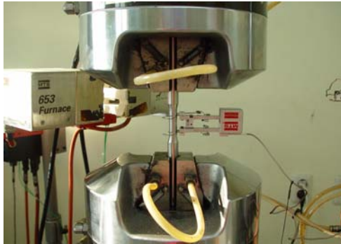
Fig. 5 Photo of MTS810 for Experiment of uniaxial tension-compression test
