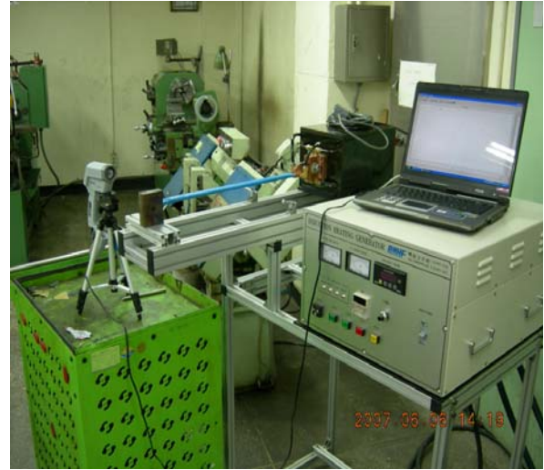
Fig. 7 Experimental setup for the induction heating
