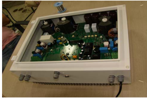
Fig. 10 Proposed 1kW PCS for fuel cell with buck/push-pull converter
