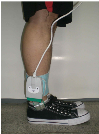
Figure 1. Sneakers and F-Scan system.
