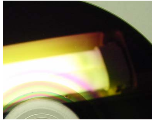
Fig. 8 Dielectric film coated NFR Media without scratch after servo tests
