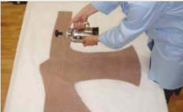
photo 21. Spray-type wet cleaning
