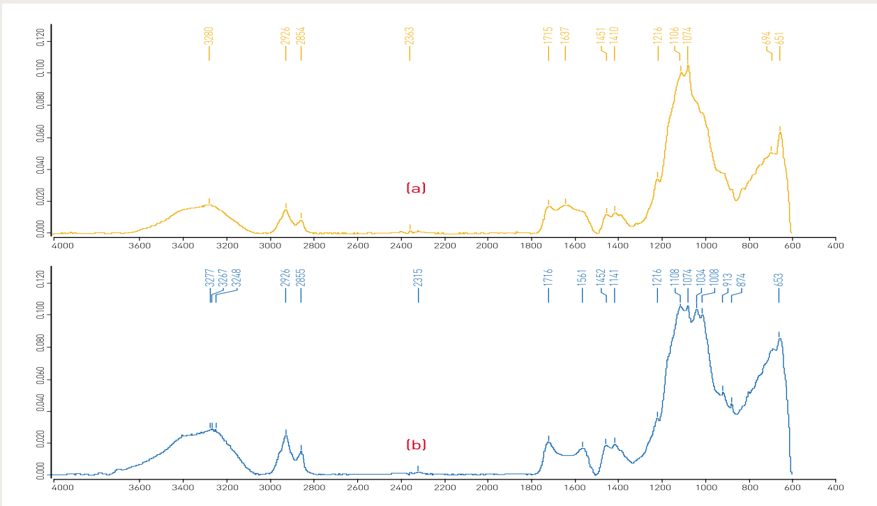
Fig. 23. Comparison adhesive material on metallic bound rim through FT-IR (a) Traditional lacquer, (b) Adhesive material in metal bound rim of Shinan2367
