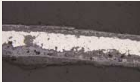
Fig. 9. Observation of Tissue Section in metal bound rim (Shinan2368)
