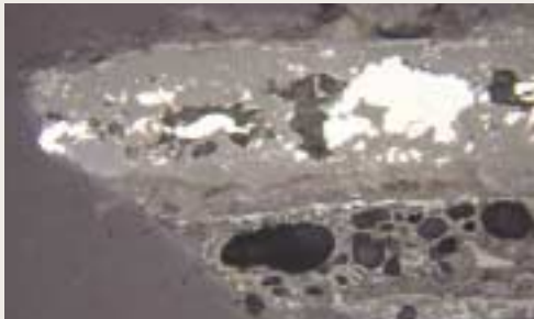
Fig. 8. Observation of Tissue Section in metal bound rim (Shinan2367)
