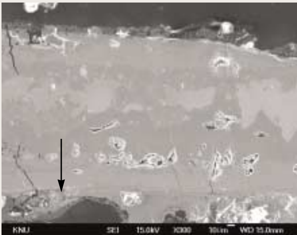
Fig. 18. Observation of metal bound rim by SEM (Shinan2367)
