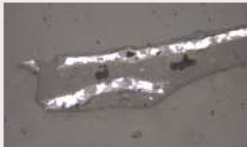
Fig. 10. Observation of Tissue Section in metal bound rim (Shinan4018)
