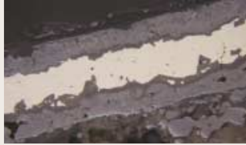
Fig. 7. Observation of Tissue Section in metal bound rim (Shinan2364)
