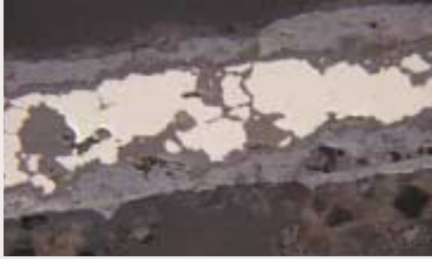
Fig. 6. Observation of Tissue Section in metal bound rim (Shinan2363)
