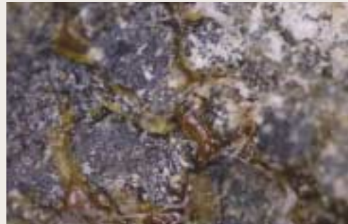
Fig. 22. Joining material of metal bound rim (X 40)
