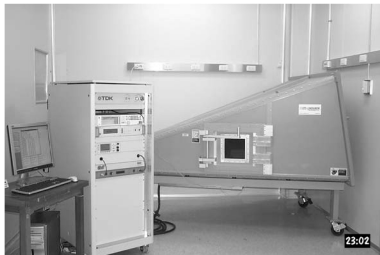
Fig. 7. GTEM system and it's circuit diagram for electromagnetic field immunity test.
