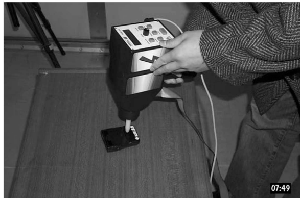
Fig. 10. Electrostatic discharge test of a Neutron personal dosimeter.
