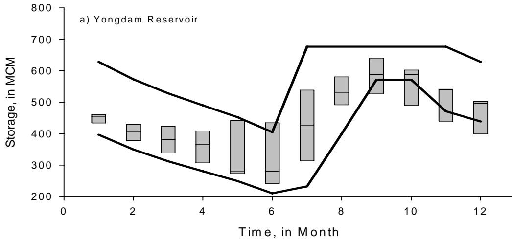
Fig. 3. General Operation Guidelines for Both Yongdam Reservoir Superimposed on Actual Reservoir Storage Levels; —: General Guidelines for Yongdam Reservoir.
