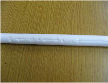
Fig. 2 Detailed sink mark for pipe
