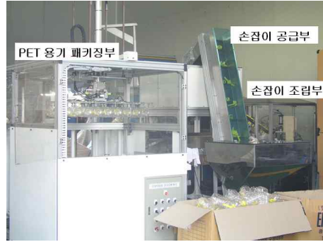
Fig. 6 Automatic packaging system of manufactured PET
