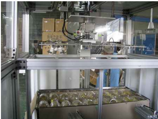
Fig. 8 Input of delivery box using jig
