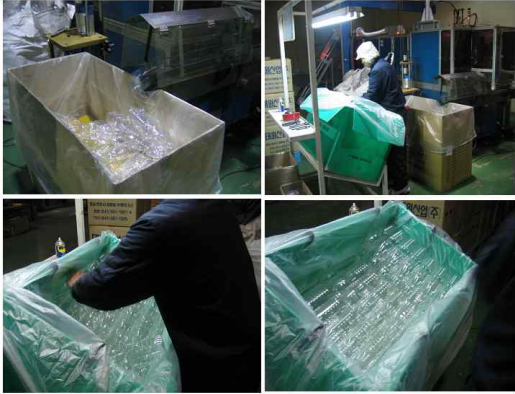
Fig. 1 General packaging process of blow molding
