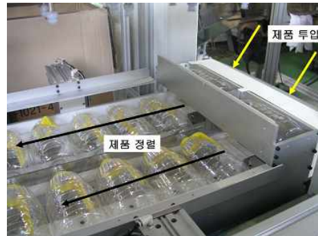
Fig. 6 Automatic packaging system of manufactured PET
