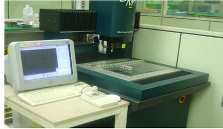
Fig.. 2-6 Laser measuring machine(De Meet
