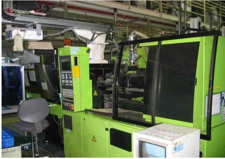
Fig.. 2-3 Injection molding machine
