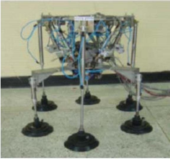
Fig. 9 ULM-IM-LLM constructed by pneumatic cylinders
