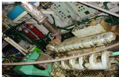
(a) Probe position for G/E NOx and smoke measurement
