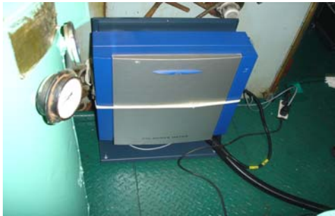
(c) AVL smoke meter
