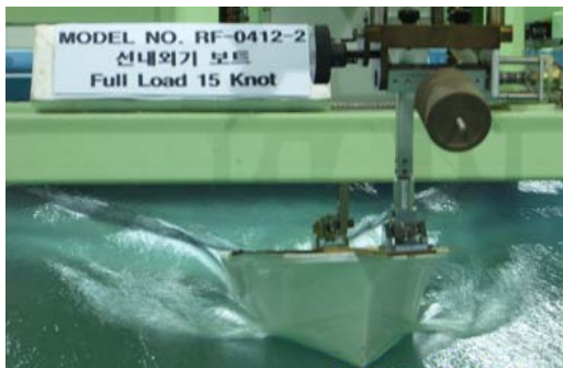
Fig. 14 Wave profile of leisure boat (In·Out-board)
