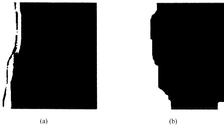
Fig. 6. Inspected binary image (a) a dye blot, (b) a unlevel dyed.
