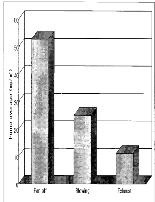
Fig. 3 Analysis result of welding fume while using the fan
