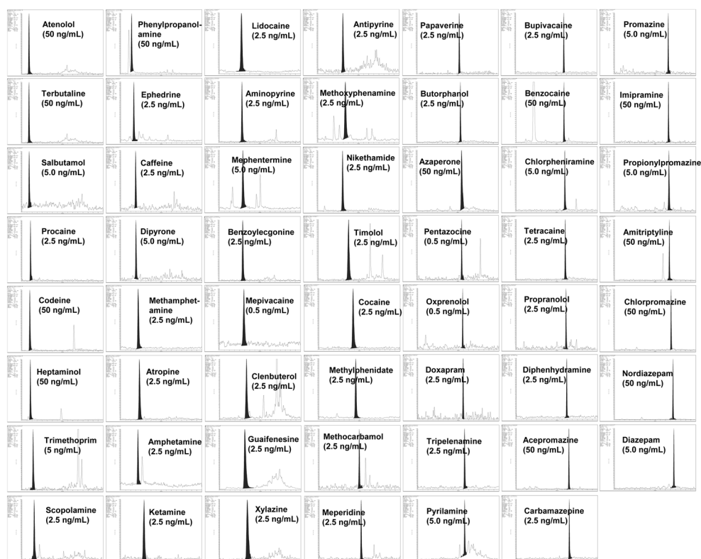
Fig. 1. Typical selected product-ion chromatograms of the 55 targeted basic drugs obtained from the analysis of spiked urine samples.
