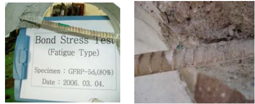
(b) Detail of Pull-out failure
