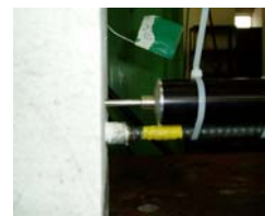
Fig. 3 Monitoring of slip test (LVDT)
