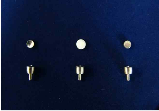
Fig. 1. Three types of magnetic attachment in this experiment (MAGFIT-IP-BFN30/BDN30/BSN30, Aichi steel Co., Japan)
