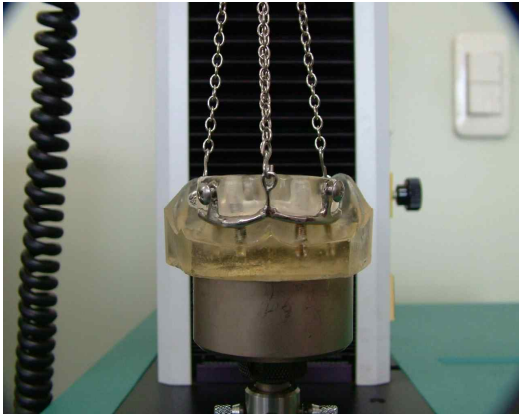
Fig. 5. The vertically directed dislodging force applied to the overdenture sample
