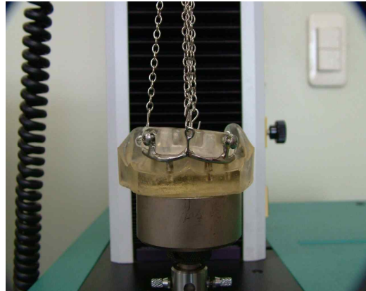
Fig. 6. The obliquely directed dislodging force applied to the overdenture sample
