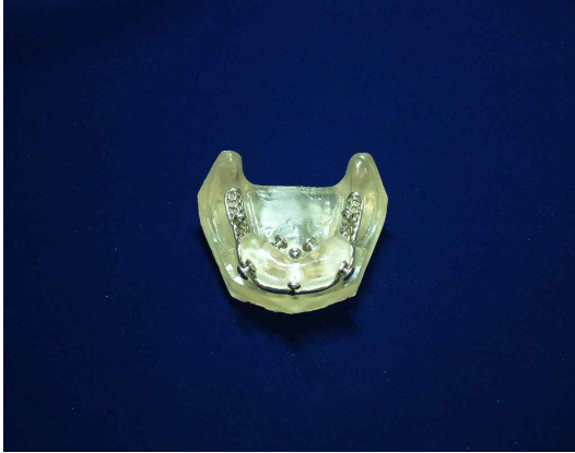
Fig. 4. Magnetic attachment overdenture sample seated on mandibular model, with nuts and bolts securely fastened
