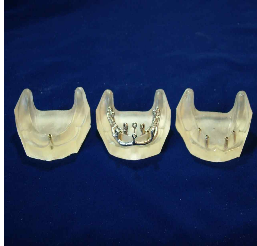
Fig. 3. Three acrylic resin mandibular models (Ortho-Jet™, Acrylic, Lang dental MFG. Co. Inc., Wheeling, USA) with single implant, two implants, four implants placed in the interforamen area and the chrome-cobalt framework with four withdrawal loops for application of tensile forces by Instron. Four 3mm-diameter
