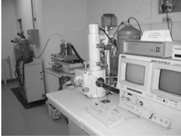
Fig. 2. SEM(JSM-5410LV, JEOL(B)).
