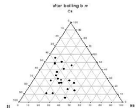
Fig. 3. Diagram of the percent cations as to property of water in bottled water.
