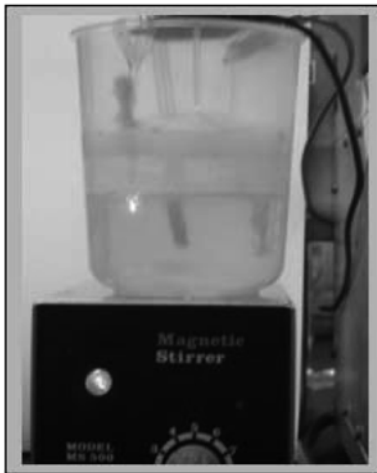
Fig. 2. Photograph of glow discharge in CGDE apparatus.
