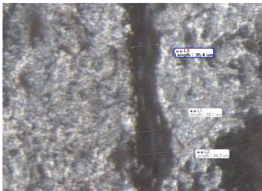
Fig. 6. Polishing specimen with pumice and tin oxide(x120)
