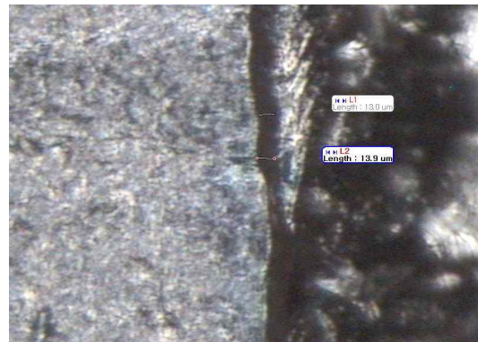
Fig. 4. Finishing specimen with FSQ-cross cut bur(x120)
