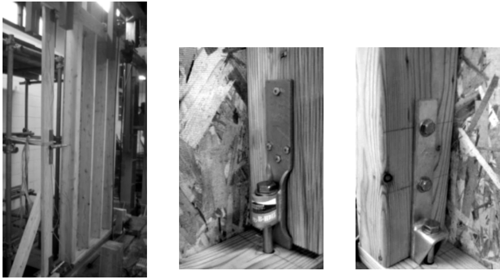
(a) Shear wall frame (b) Applied B-HD hold-down (c) Applied S-HD hold-down
