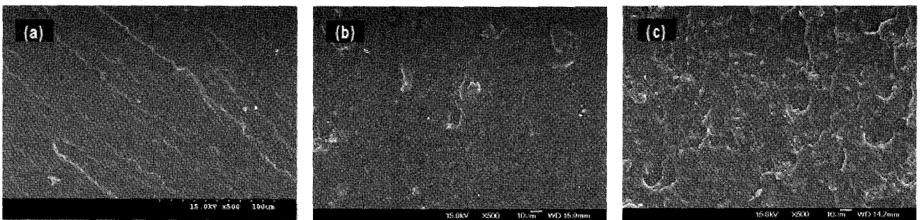
Figure 10. SEM image of fracture surface of CTBN toughened epoxy/Cloisite 30B nanocomposite with different MMT content. (a) 0, (b) 5, and (c) 15 phr ( \times 500 ).
