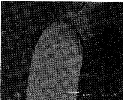
(c) PP/PP- g -MAH/ no-surface treatment PET fiber=95/2.0 (phr)/5
