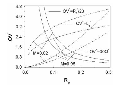
FIGURE 4. Optimum values versus the fin outer radius ( $L_b=0.1$ ,  $\beta=1$ )
