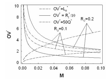
FIGURE 6. Optimum values versus ambient convection characteristic number ( $L_b=0.1$ ,  $\beta=1$ )
