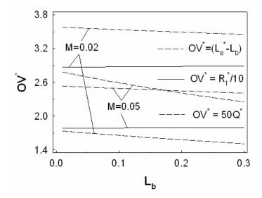
FIGURE 3. Optimum values versus the fin base thickness ( $R_0=0.15$ ,  $\beta=1$ )
