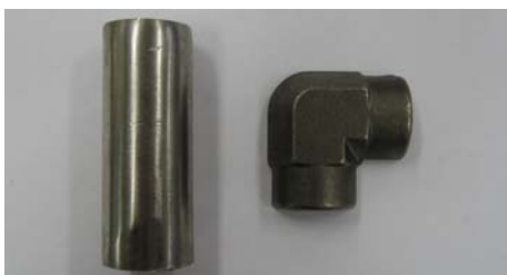
(a) initial billet by the developed process and its product
