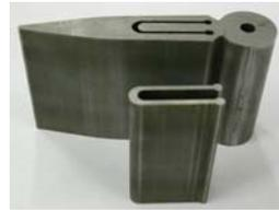
Fig. 1 Compound dies (blanking & piercing)
