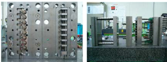
Fig. 16 8-cavity die for injection molding of camera module holder
