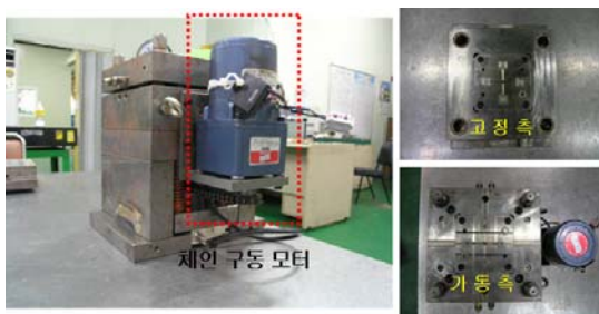
Fig. 10 Die set with chain-driven ejecting mechanism
