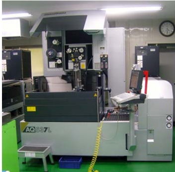
Fig. 7 CNC EDM(Electro Discharge Machining)
