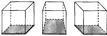
Fig. 2. Three cases of the projected shape for a rectangular parallelepiped object. Red bold lines represent base edges and blue bottom rectangles base shapes.
